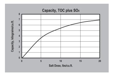
**CAPACITY** — The graph above is based on 2 gpm/cu.ft. flow rate, pH near neutral, and 36 inch minimum bed depth. Capacity is for TOC plus sulfate. No engineering downgrade has been applied.
