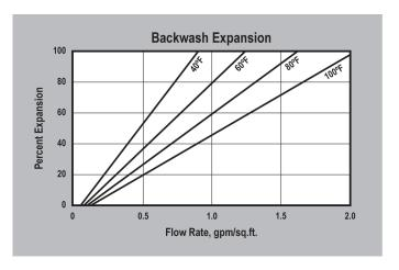
**BACKWASH** — After each cycle the resin bed should be backwashed at a rate that expands the bed 25 to 50 percent. The graph above shows the expansion characteristics as a function of flow rate at various temperatures.
